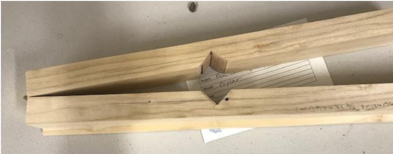
Bill Johnson developed this holding device for drilling pen blanks on his drill press. There is a hinge on one end, and you place the blank in the holder and drill away. Helps is blanks are the same size.
