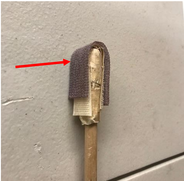
This is how Susan sands the inside with Abranet on a stick
