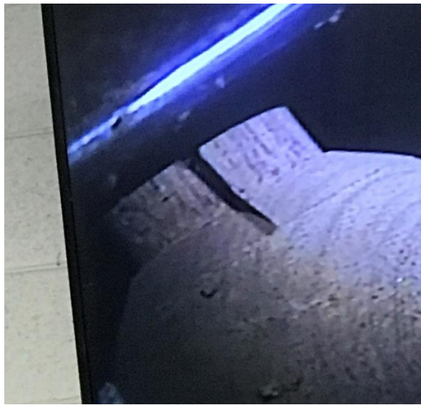
Marks by parting tool to aid in rounding sphere
