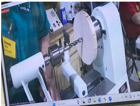
He then reverse chucks the piece and drills a 5/8 " hole and then shapes the front
