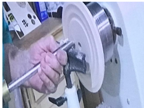
He then reverse chucks the piece and drills a 5/8 " hole and then shapes the front
