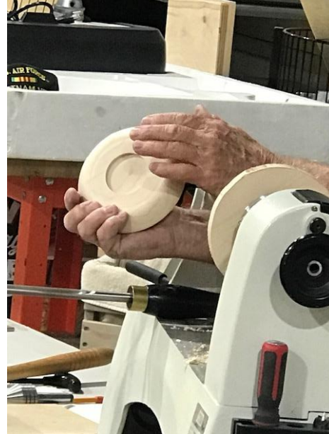
Connis uses Cole jaws to put the reverse tenon on the piece
