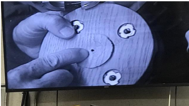
The donut clamp with Scott showing starting hole
