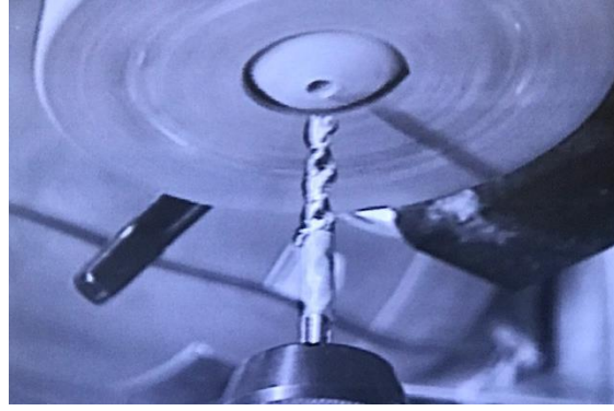
Drilling hole in ball to start the hollowing process. Tape indicates the maximum depth of the drilling.
