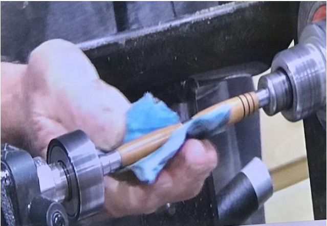
After sanding the turned pen blank to 400 he applies friction polish with paper towels. He stated that you run it until it is hot.
