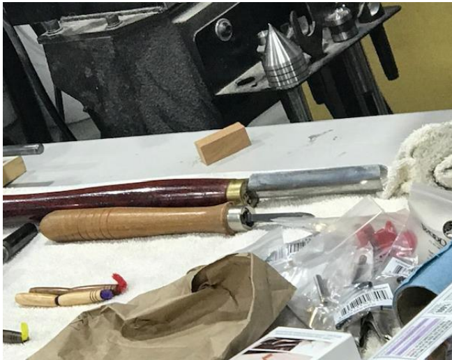
These are the tools that Connis uses to turn the blank. He starts out with the roughing gouge and then uses a skew to do the final cuts.
