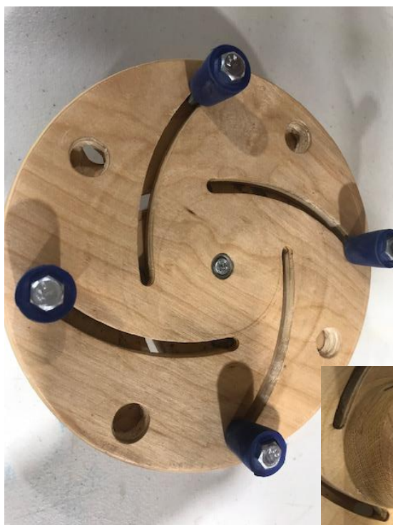
Sid Bright's handmade chucks similar to Cole Jaws. The back is designed to screw onto the headstock
