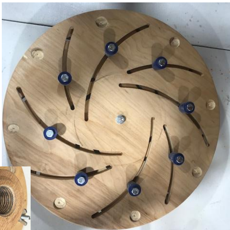
Sid Bright's handmade chucks similar to Cole Jaws. The back is designed to screw onto the headstock
