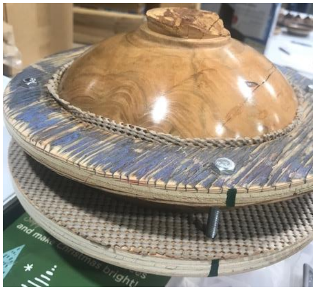
Sid Bright's donut chuck. Depending on the size of the bowl he changes out the circle. This will allow him to work the bottom of the piece.
