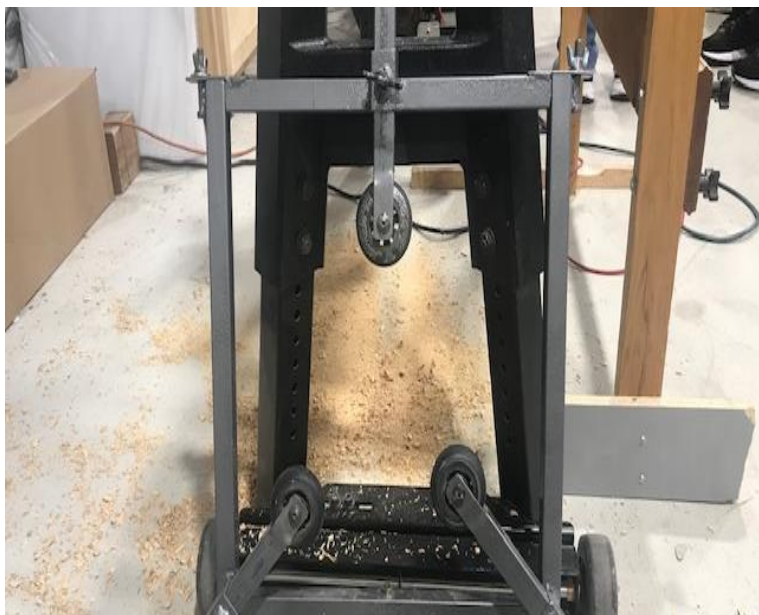
This is the unit that Sid developed out of metal. The top has wing nuts and can be taken off so you can put it over a piece that is mounted on the lathe. There is a plate on the bottom that allows him to attach it to his lathe.
