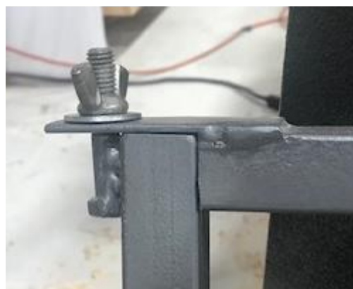
This is the unit that Sid developed out of metal. The top has wing nuts and can be taken off so you can put it over a piece that is mounted on the lathe. There is a plate on the bottom that allows him to attach it to his lathe.
