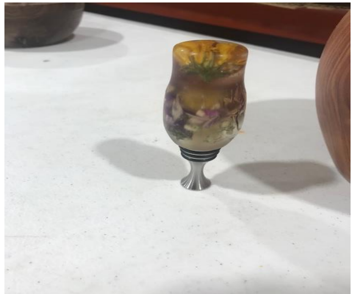
Resin cast flowers as a bottle stopper by Rob Lucas. He is working on how to cast the flowers. Has had some voids. Clear Cast materials
